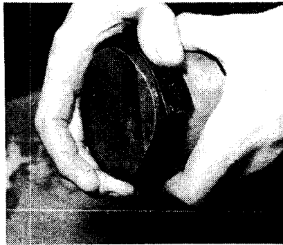
45.9A Fitting a piston ring clamp
