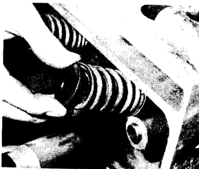
12.5A Removing valve top cup and spring
