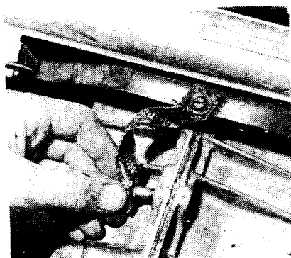
5.17 Disconnecting an earthing strap
