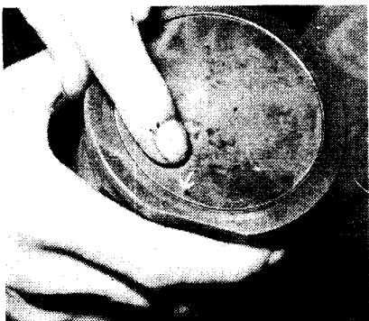
45.9C Piston crown directional arrow (faces front of engine)
