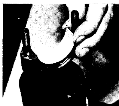
45.2 Fitting a big-end bearing shell
